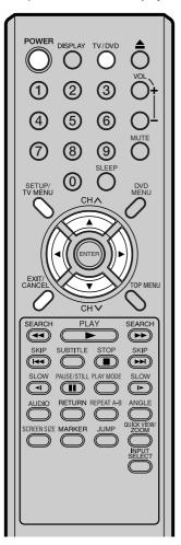
**1** Press **POWER** to turn on the unit. 2 Press **TV/DVD** to select the TV mode. 3 Press **SETUP/TV MENU**. The TV menu screen will appear. 4 Press ◀ or ► to select 💾 (SETUP) menu. Ģ SETUP LANGUAGE ENGLISH CLOCK SET TV/CABLE AUTO CH MEMORY ADD/DELETE CABLE .SELECT :ADJUST 5 Press ▲ or ▼ to select "LANGUAGE". K SETUP LANGUAGE ENGLISH ENGLISH/FRANÇAIS/ESPAÑOL CLOCK SET CABLE AUTO CH MEMORY ADD/DELETE AUTO :SELECT ADJUST
